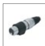
S.3497 XLR5 TERMINATOR with integrated 120 Ohm resistance. To be used as termination of DMX line for item S.1066 IP65
