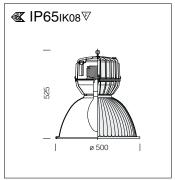
Housing: die-cast aluminium with wide cooling fins.
