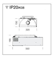
Housing: made of sheet steel galvanised and coating.
